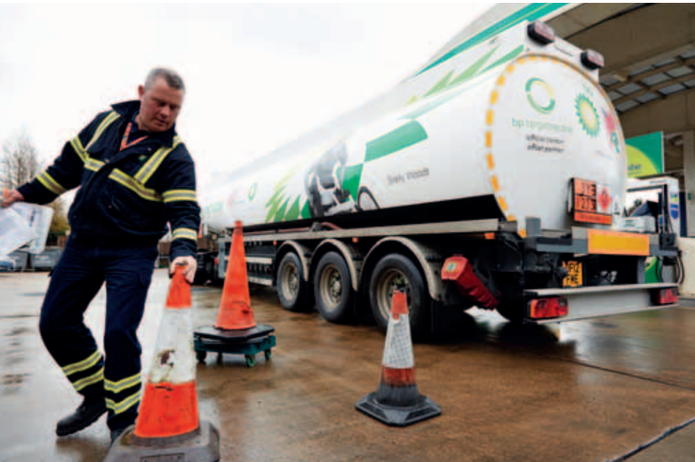
Forecourt delivery: good customer relationships are key. Left, Jeremy fills out his delivery paperwork with the assistance of the station’s competent person; above, Jeremy cones off a safe delivery area, as described in the delivery risk assessment. The Hazchem panel – the orange rectangle – is clearly visible on the rear of the tanker; and right, Jeremy connects the vapour recovery hose at the service station.
