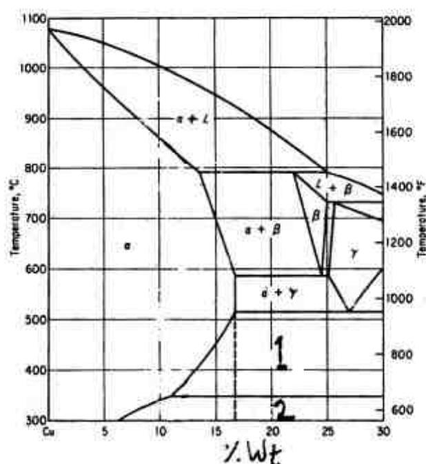
$\gamma = \alpha + \delta$ ,  $\gamma = \alpha + \varepsilon$ , Cu-Si (۱) $\gamma = \alpha + \varepsilon$ ,  $\gamma = \alpha + \delta$ , Cu-Al (۲) $\gamma = \alpha + \delta$ ,  $\gamma = \alpha + \varepsilon$ , Cu-Zn (۳) $\gamma = \alpha + \varepsilon$ ,  $\gamma = \alpha + \delta$ , Cu-Sn (۴)
